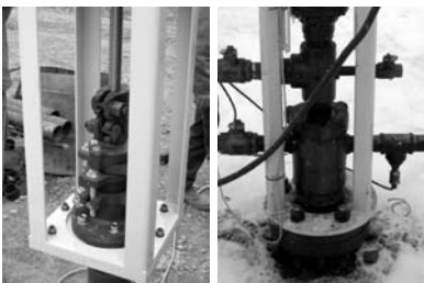
The unit installs quickly and mounts directly to the stuffing box or well casing
