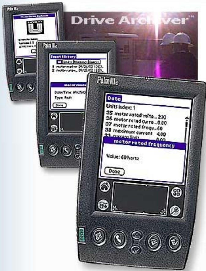
The Drive Archiver ™ Data view shows all parameters and their values. The Events History screen lists all drive faults, warnings, and events along with the date and time they occurred.
