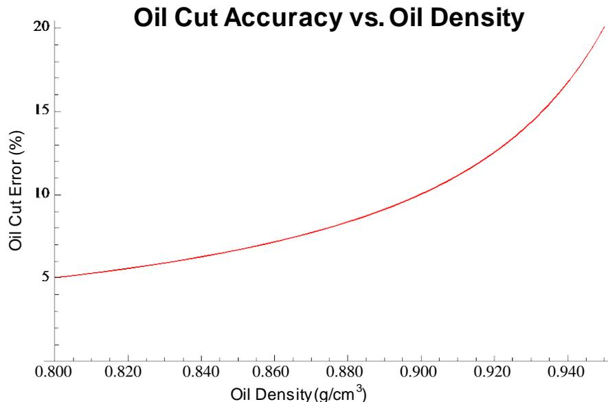
**Fig. 1:** Plot of the percent error in the oil cut vs. the density of oil, based on the  $\pm 0.001 \text{ g/cm}^3$  accuracy of the meter's density measurement. This graph assumes a 10% oil cut with water density equal to  $1.0 \text{ g/cm}^3$  and no free gas present. As the difference between the oil and water density decreases the error increases.
