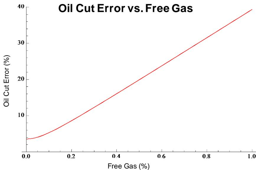
**Fig. 3:** Plot of the percent error in the oil cut vs. the percent of the fluid volume occupied by free gas (0 – 1% free gas). This graph assumes a 10 % oil cut with oil density equal to  $0.823 \text{ g/cm}^3$  and water density equal to  $1.105 \text{ g/cm}^3$ .
